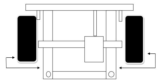
Wheel track measurement points front and rear 43" - 45"
