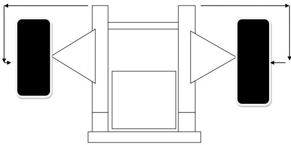
Rear end tech off set measurement points 0" - 1/2" or 0mm-12mm
